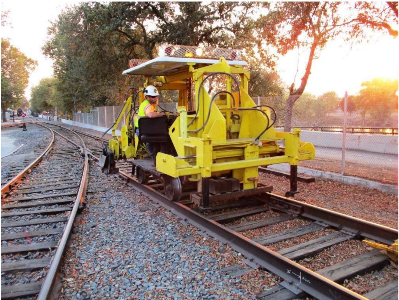
Joe takes out the Jackson 125 tie-exchanger as part of the “almost” big move
