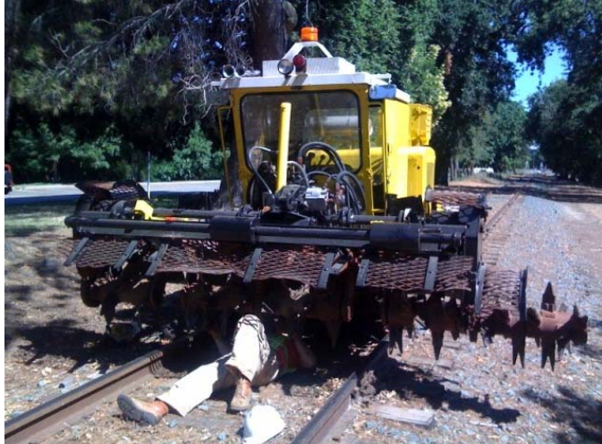
Mike performing field repair to the scarifier prior to use in the tie change out project.
