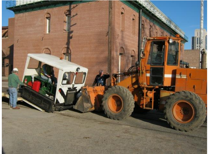
The loader is used to give a little extra help to load one of the broken motor cars onto the trailer to be hauled back to the shop for repair.
