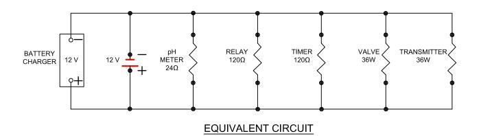
The equivalent circuit shows all the various components connected to the system in parallel which provides a very simple way to analyze the circuit further if you wanted to know the amount of power being consumed, for example
